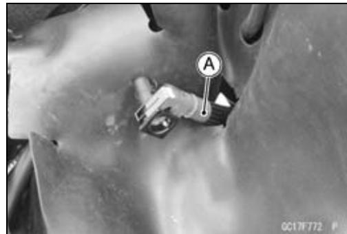
○ To maintain the correct fuel/air mixture (F/A), there must be no intake air leaks in the DFI system. Be sure to install the oil filler plug [A] after filling the engine oil.
