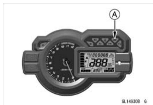
★ If the meter is good, check the wiring continuity of the Y lead in the main harness.
