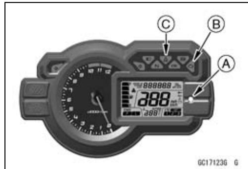
The self-diagnosis system has two modes and can be switched to another mode by operating the meter unit.
